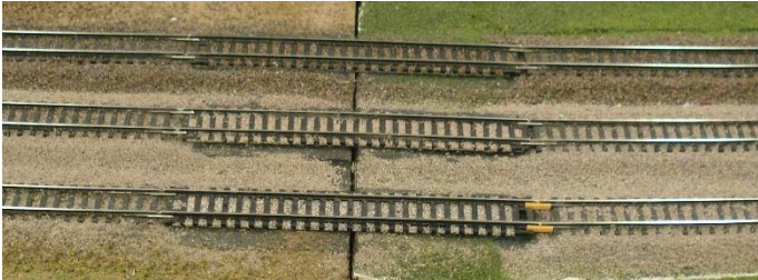
Regular Joiner Track with Insulated Joiner on bottom and middle tracks, and regular joiner on top track
